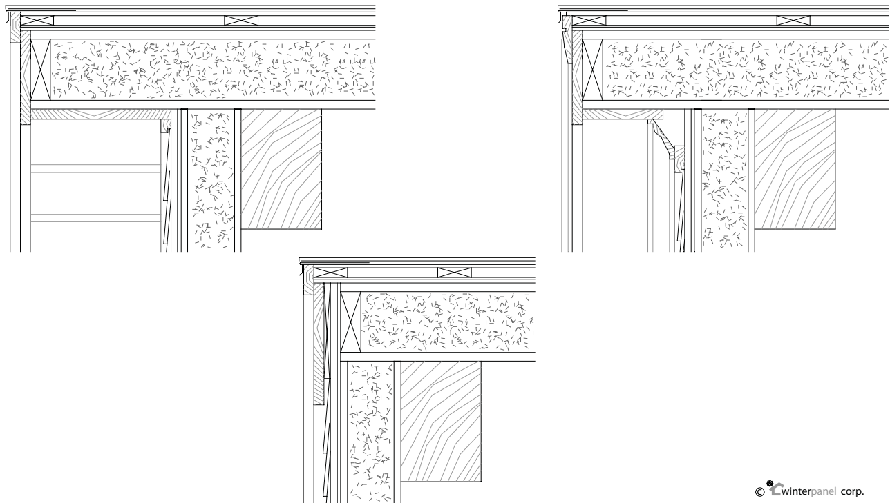
Figure 69. Trim Options at Gable. Several options for trim at the gable end roof edge are shown here. The trim can be as simple or ornate as desired.
